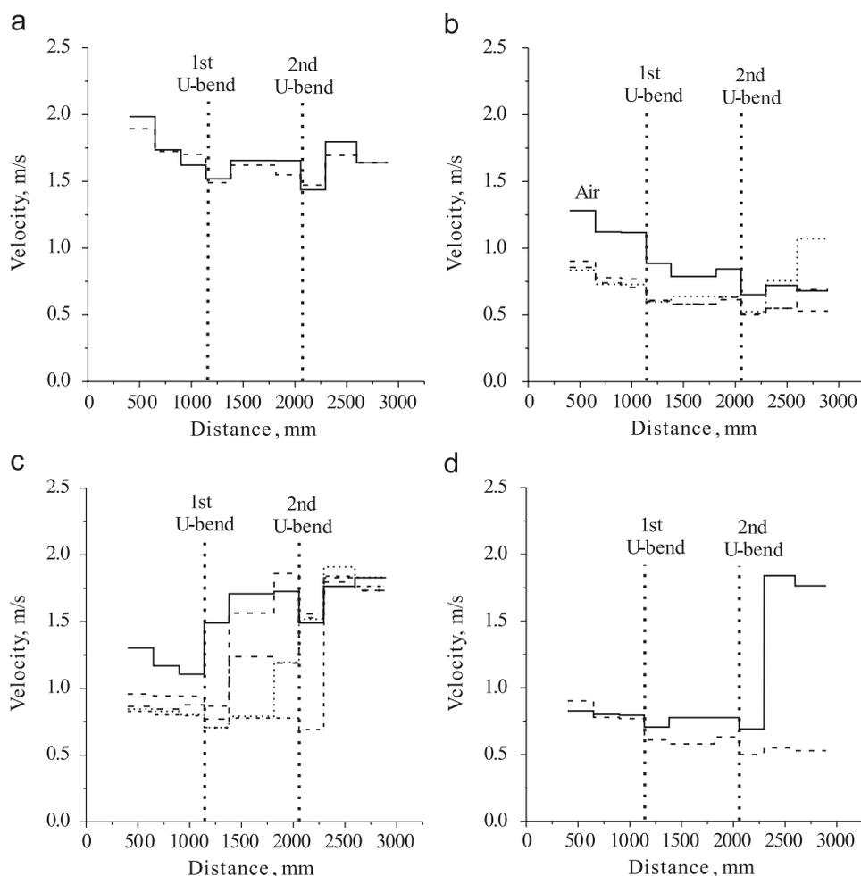
Fig. 4. Mean shock wave velocities at different measuring segments of the tube with two U-bends (shown by vertical lines) in some representative runs: (a) transition of detonation through two U-bends, (b) transition of shock waves through two U-bends without detonation onset, (c) transition of shock waves through two U-bends with detonation onset, and (d) phenomena in the vicinity of the critical primary shock intensity.
