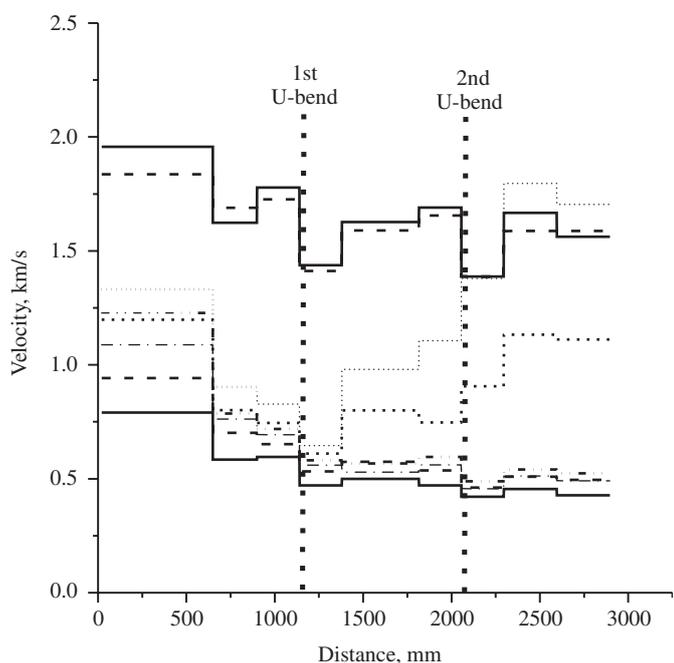
Fig. 6. Mean shock wave velocities at different measuring segments of the tube with two U-bends (shown by vertical lines) in some representative runs with electric-discharge SG.
