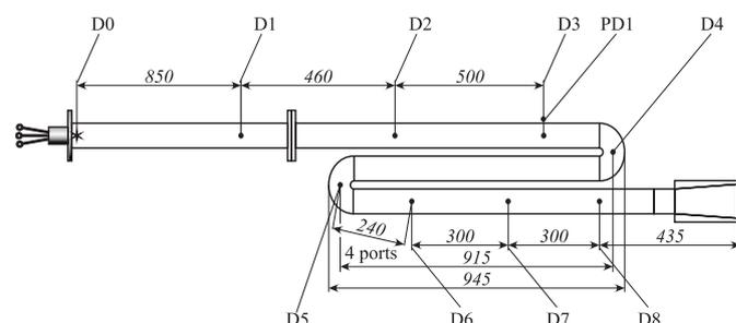
Fig. 3. Experimental setup with the electric-discharge SG and with the elongated initiation section. PD1 stands for photo-diode. Dots indicate the positions of pressure transducers (see Table 3).
