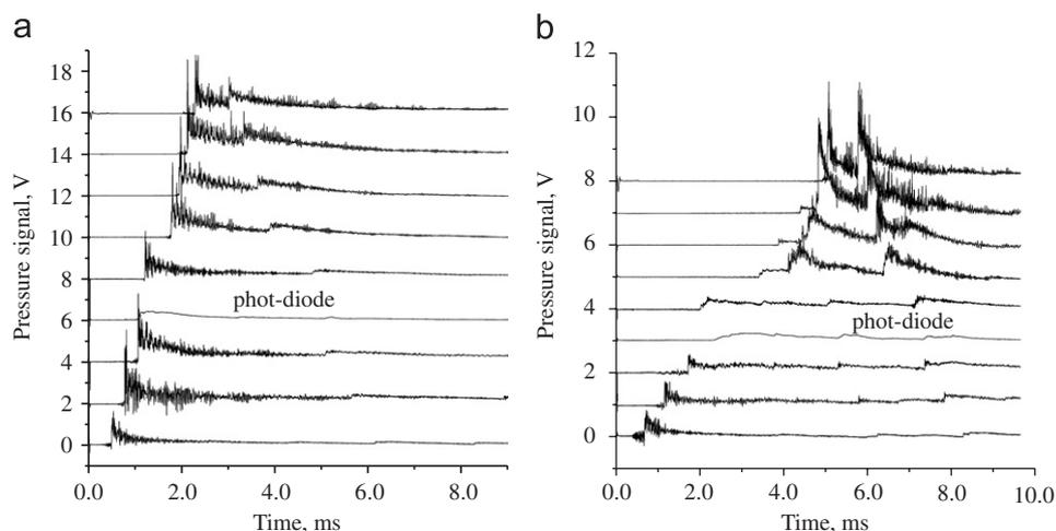
Fig. 9. Representative pressure records: (a) detonation with the photo-diode in the same cross-section with D3 and simultaneous signal; and (b) no shock-to-detonation transition with the time delay of photo-diode activation.
