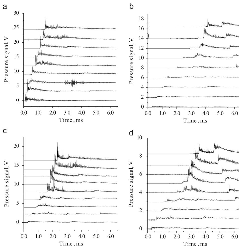
Fig. 5. Pressure records: (a) detonation, (b) shock wave with a strong pressure wave in the wake, (c) SDT, and (d) shock wave with the strong pressure wave catching up with the lead front.
