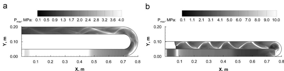
Fig. 10. Predicted fields of maximal pressure at identical conditions of shock wave generation in tubes with different U-bend curvature: (a) no detonation, and (b) detonation.
