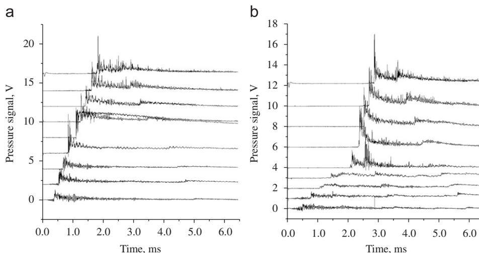
Fig. 7. Pressure records: (a) detonation; and (b) SDT.
