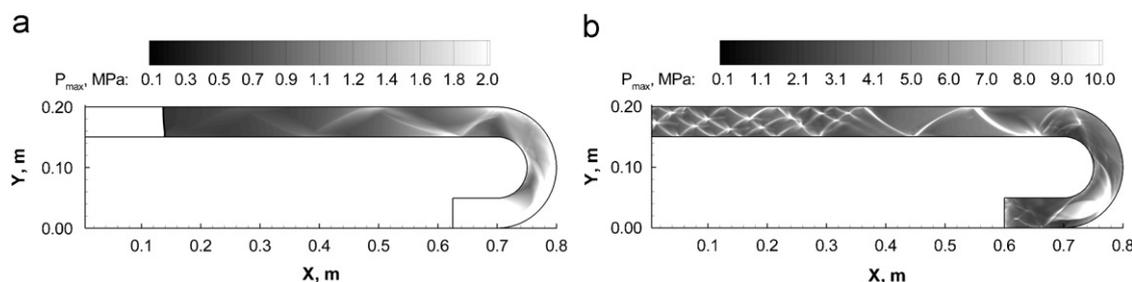
Fig. 11. Predicted maximal pressure field in the course of primary shock wave propagation in the tube with U-bend. Initial shock velocity is 1460 m/s; compression phase duration is 30  $\mu$ s (a) and 50  $\mu$ s (b). In the left figure, the shock wave decays, in the right figure the shock wave initiates detonation.
