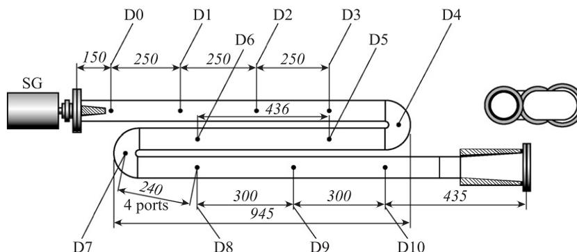
Fig. 1. Schematic of the experimental setup with the solid-propellant SG. Dimensions are in millimeters. Dots indicate the positions of pressure transducers (see Table 1).
