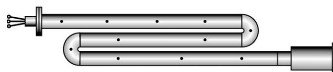
Fig. 2. Experimental setup with the electric-discharge SG. Dots indicate the positions of pressure transducers (see Table 2).
