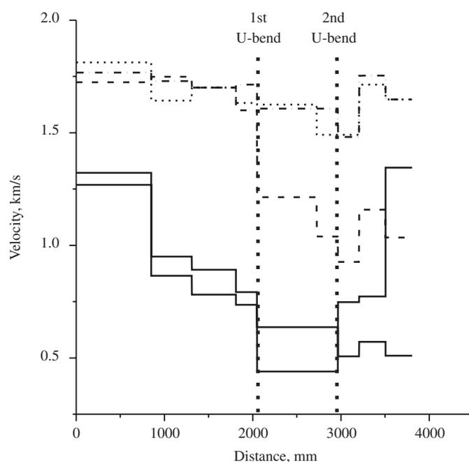
Fig. 8. Mean shock wave velocities at different measuring segments of the tube with two U-bends (shown by vertical lines) in representative runs.
